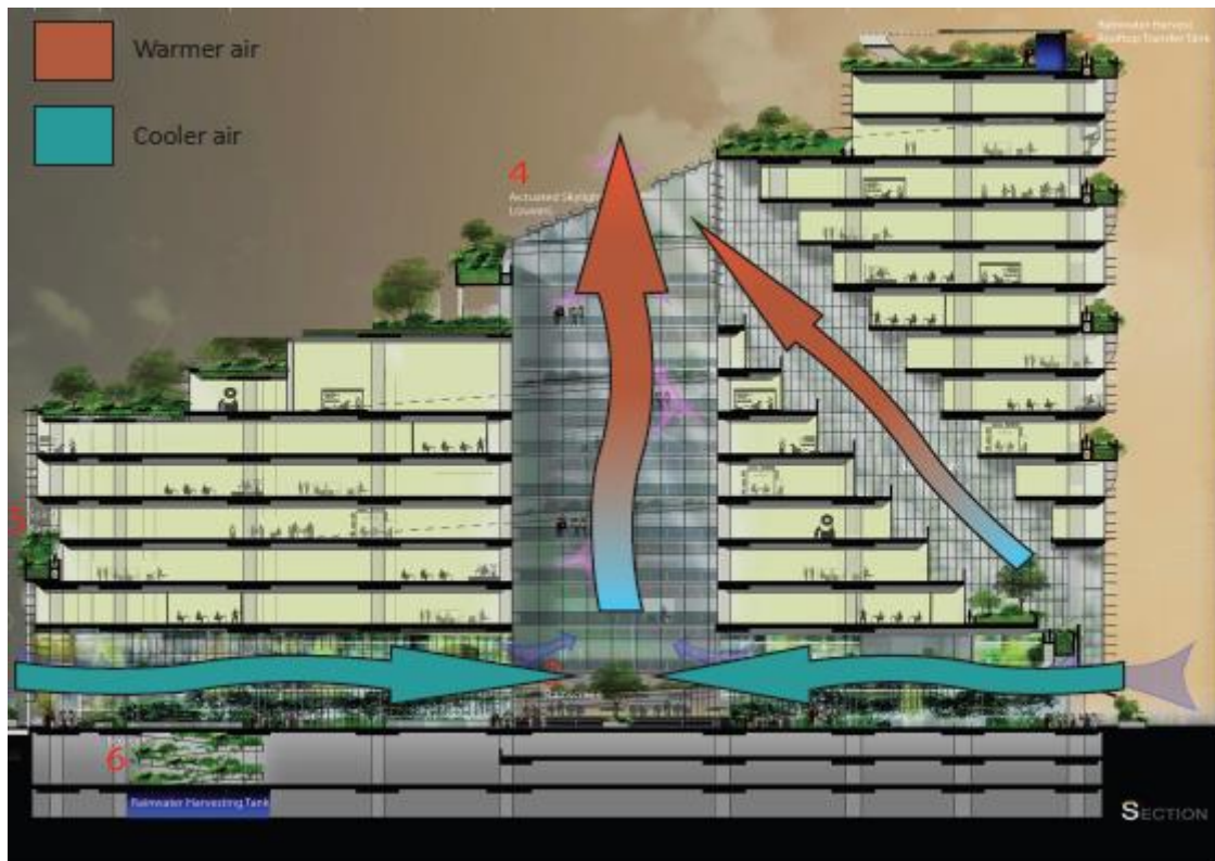
Figure 15: Section shows the flows of air circulation throughout the atrium, stack ventilation (Source : http://blog.cpgcorp.com.sg/wp-content/uploads/2012/03/Solaris_Section.jpg )
